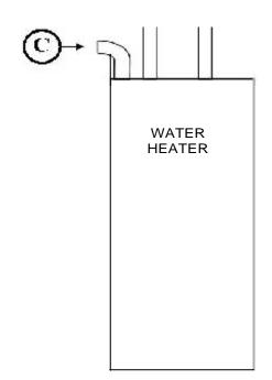
Open relief valves prohibited. These must be piped to the drainage system or to another safe location, such as the floor [the open end of which can be no more than six inches (6") above the floor].
